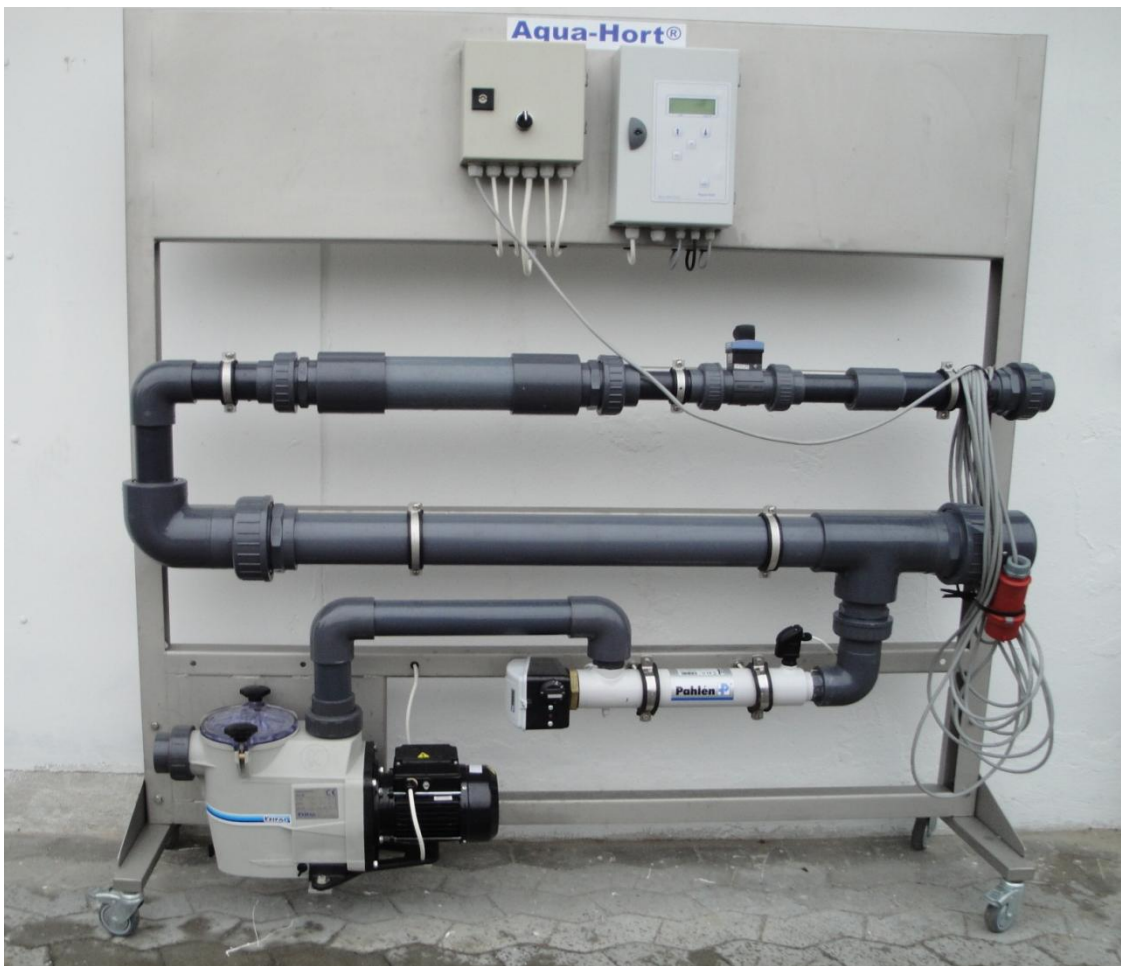
Picture 1: Below pump and electric heater. Second row Aqua-Hort electrode. Third row electromagnet and flow meter
